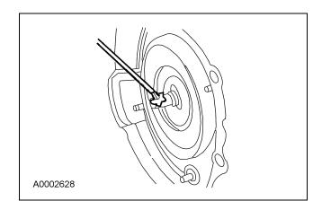
In order to correctly install the special service tool, it must be installed using one round and one oblong hole. Using two oblong holes will cause damage to the transmission.
